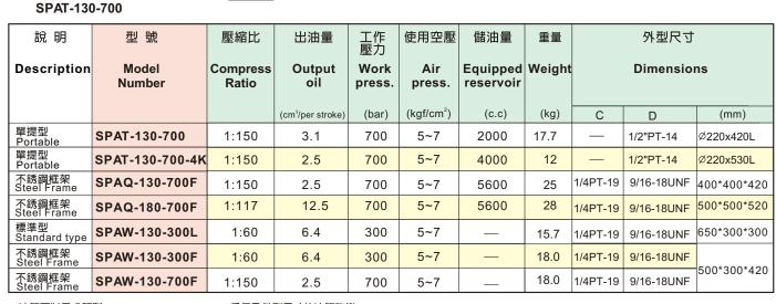
※油箱可以需求訂製 \*Reservoir will be changed by user ※重量及外型尺寸依油箱改變 \*Weight and dimension will be changed by reservoir alter.
