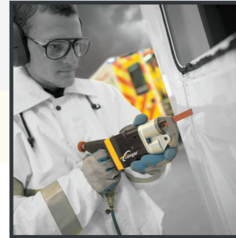
Steel Sections Bolts, Gratings etc. up to 6mm thick and 25mm Composites.
